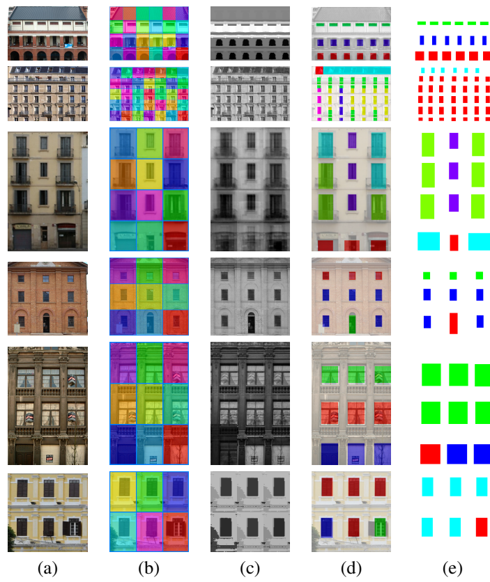
Figure 3: (a) Input image, (b) detected partitions, (c) low-rank component, (d) detected repeated patterns, and (e) ground truth.
