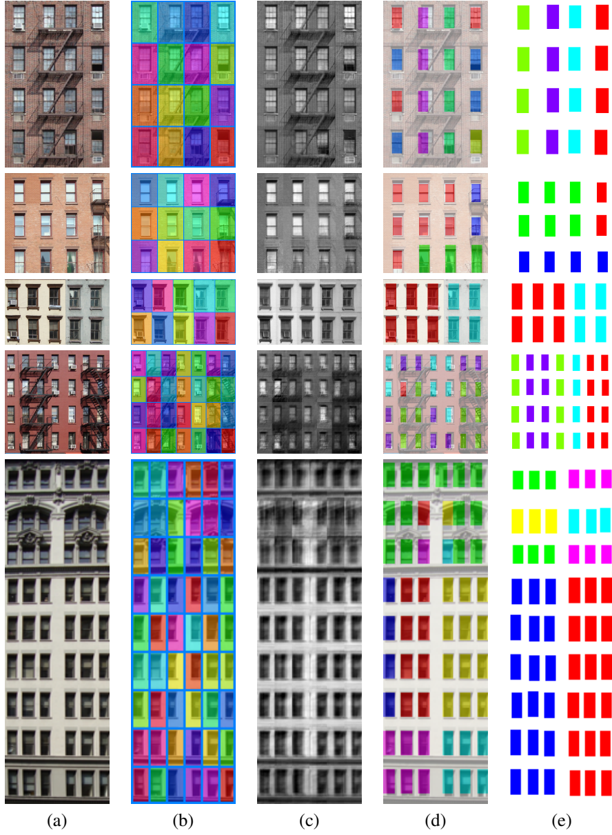
Figure 6: (a) Input image, (b) detected partitions, (c) low-rank component, (d) detected repeated patterns, and (e) ground truth.
